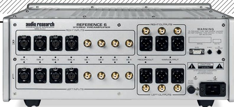
**ABOVE:** Line-level preamp offers four balanced (on XLR) and four single-ended (on RCA) inputs with pairs of XLR/RCA outputs (plus rec out). RS232 services automation
