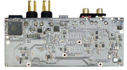
Much of the circuitry is associated with the all-important Xilinx FPGA chip. A 32-bit ARM-based Atmel microcontroller looks after the Qutest's operation, and provides its USB interface.
