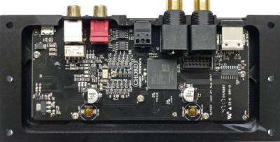
Substantial machined casework and meticulous circuit board. An obvious part of the latter is the large FPGA chip on which Rob Watt's DAC is implemented.
