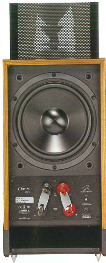
The rear 8in aluminium cone bass unit works in a chamber loaded by a slot-port at floor level. Bi-wiring is possible. A small d.c. power input and blue LED are sited here too.
