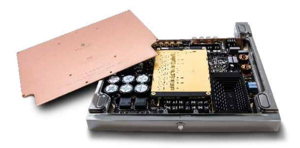
▶ It's effectively added 50% more power to the previous models, and includes more filter inductors per channel. The analogue to digital conversion stage (Magic Wire in Devialet-speak) is new, too, knocking 6dB off the THD and cutting the noise floor by 2.5dB. Add in a power supply that can now deliver 4kW and a very sophisticated (and large) thermal management system, which includes a 2.5kg copper base plate, and it all becomes clear that this is not simply old wine in new bottles.
