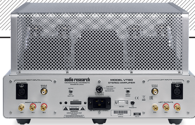
ABOVE: Balanced (XLR) and single-ended (RCA) inputs are selected by a toggle and separate 8/4ohm speaker taps are offered on 4mm terminals. Note the 15A blade-style mains inlet and second toggle to facilitate auto shut-off, preserving valve life
