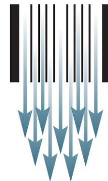
Turbulent airflow at the ATL™ vent without Laminair™
