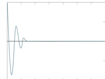
The diagrams above show how unwanted cabinet vibrations, left untreated, continue to resonate and distort speaker output, and, by comparison, how the vibrations are cancelled by mass damping in fenestria.
