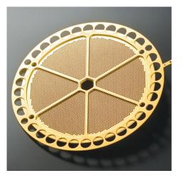
electrode itself. Reducing vibrations and ringing to a minimum. The sound quality has been further improved by lowering the resistance of the electrode as well. In addition, the holes on the electrode are precisely placed, ensuring smooth sound permeation.
