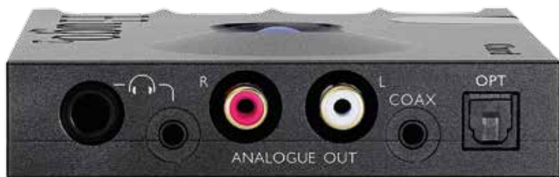
ABOVE: Conventional digital ins and analogue outs are all grouped on one end of the Hugo 2, with new high-quality labelling: both 3.5mm and 6.35mm headphone outs are provided, plus line audio on RCAs and optical/coaxial digital inputs
