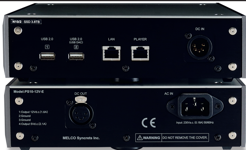
ABOVE: Melco offers network and direct player Ethernet connections from the player [upper] plus two USB-A ports, one to drive a USB DAC and one to connect an (expansion) USB HDD. The 5-pin XLR carries 5 / 12V DC from the PSU [lower]
