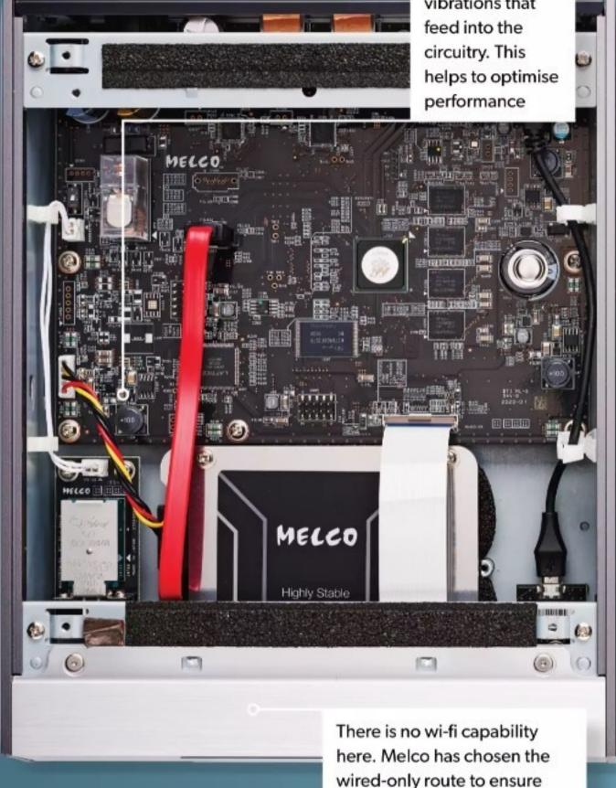
The N10/2 has an outboard power supply to minimise any unwanted interaction between the sensitive audio circuits and the high currents flowing in the supply section. It is interesting that Melco has decided to go for a traditional linear design rather than the more usually seen switch-mode type
