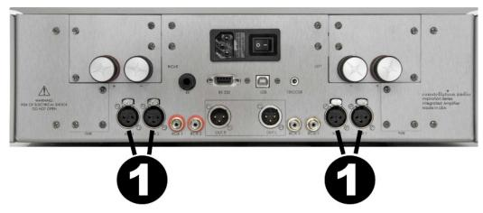
On the rear of the Inspiration Integrated are four XLR inputs, two on each side. As you are looking at the rear panel, the left two XLR inputs are for the right channel, the right two inputs are for the left channel. Underneath each jack is the corresponding input number. Use of XLR connections is recommended for the best possible audio quality. To remove an XLR plug, push on the tab above the jack and pull the plug out.
