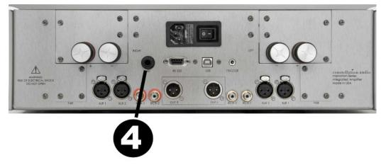
The Inspiration Integrated offers a single headphone output on a 1/4-inch (6.2mm) jack. To activate this output (and mute the speaker outputs), you must use the front-panel controls. The Inspiration Integrated's headphone amplifier has enough power to drive any dynamic or planar magnetic headphones. If your headphones have a 1/8-inch (3.5mm) plug, use a 1/8-inch to 1/4-inch adapter. Many headphones come with the adapter.
