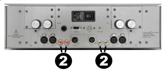
These unbalanced inputs are provided as a convenience for use with unbalanced signal sources. Whenever possible, we recommend using XLR connections instead. Connecting to an unbalanced source is handled in the same way an XLR balanced source. To remove an RCA plug, grasp the plug and pull it out. Do not pull on the cable.
