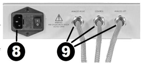
Each of these cables mates with a matching jack on the preamp. Be sure to connect the Analog Right power cable from the supply to the Analog Right jack on the preamp, the Analog Left power cable from the supply to the Analog Left jack on the preamp, and the Control power cable from the supply to the Control power jack on the preamp.
