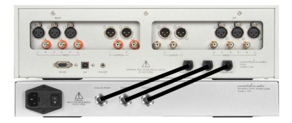
The Pictor's separate power supply (bottom component in the picture above) must be connected to the Pictor main chassis (top component in the picture above) as shown above before you plug the unit into a wall. Make sure the power switch on the power supply is in the off (O) position. The supplied cables are spiral-wrapped, gold-plated copper designed for aerospace use, and can handle up to 30 amps. Only these cables should be used between the power supply and the Pictor.
