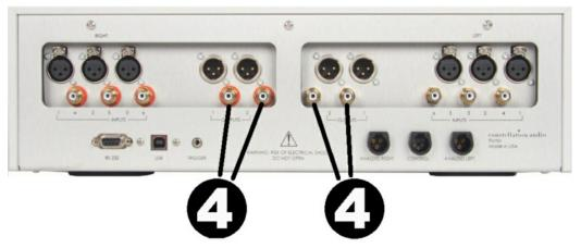
RCA unbalanced outputs are also supplied for amps and recording devices not equipped with XLR jacks. The signal at these outputs is the same—it does not matter if you use output 1 or output 2.
