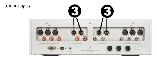
The inner XLR connections on the rear of the Pictor are outputs. The signal at these outputs is the same—it does not matter if you use output 1 or output 2. To remove an XLR plug, push on the tab on the connector body and pull the plug out.
