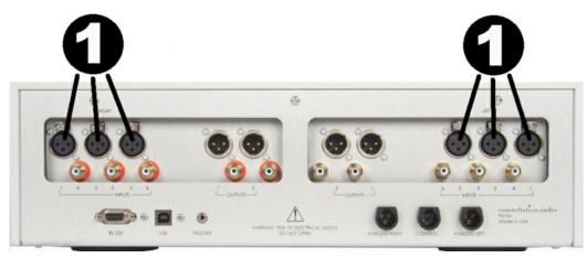
On the rear of the Pictor are six XLR inputs, two on each side. As you are looking at the rear panel, the left three XLR inputs are for the right channel, the right three inputs are for the left channel. Underneath each jack is the corresponding input number. Use of XLR connections is recommended for the best possible audio quality. To remove an XLR plug, push on the tab above the jack and pull the plug out.
