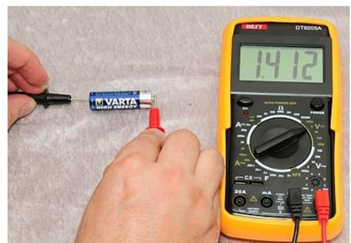
There are *always two points* in any voltage measurement: a reference point and another point in the system.
