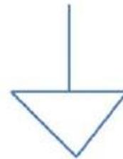
FIGURE 1: Signal ground symbol.
