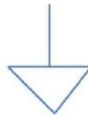
FIGURE 1: Signal ground symbol.
