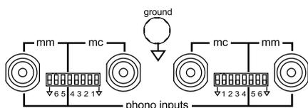
The phono inputs are balanced. Setting the ground switch ↓ to the up position references the input to ground which is sometimes useful if there is excessive noise or hum present.
