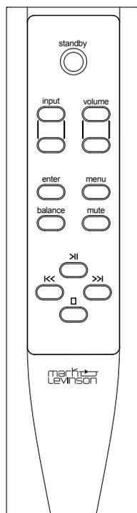
**Standby:** Press this button to put the N°5805/ N°5802 into and out of the *Standby* mode. Press this button twice to wake up unit from green *Standby* mode.
