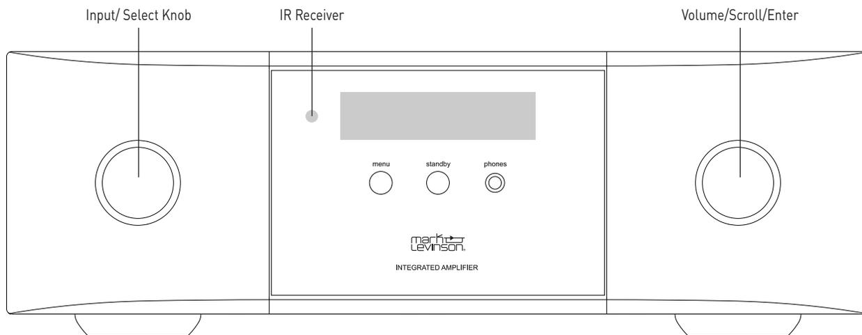
The N°5805 / N°5802 was designed for elegant simplicity and ergonomics. Therefore the knobs perform a variety of functions depending on the operating mode. There are two modes of operation, Listening mode and Setup mode, and three modes of standby, Green, Power-save, and Normal.
