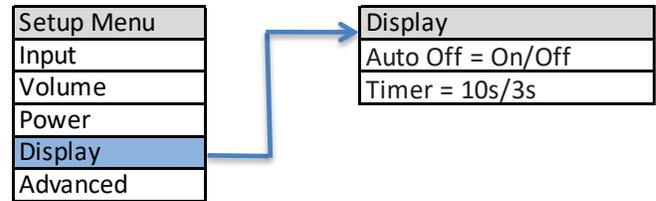
The Display function allows you to choose whether the front panel display stays on all the time, or turns off after a selectable amount of time.
