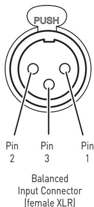
Balanced connector pin assignments:
