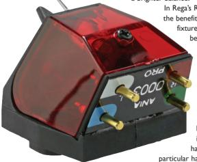
Widely spaced rear signal pins, unobstructed by body overhang, make connection easy. Clear colour coding, Right channel (+red/-green) and Left channel (+white/-blue) help get things right.
