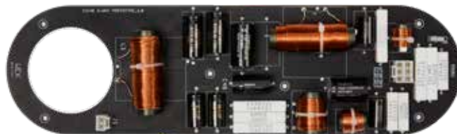
The hand-built three-way ci140 precision crossover.
