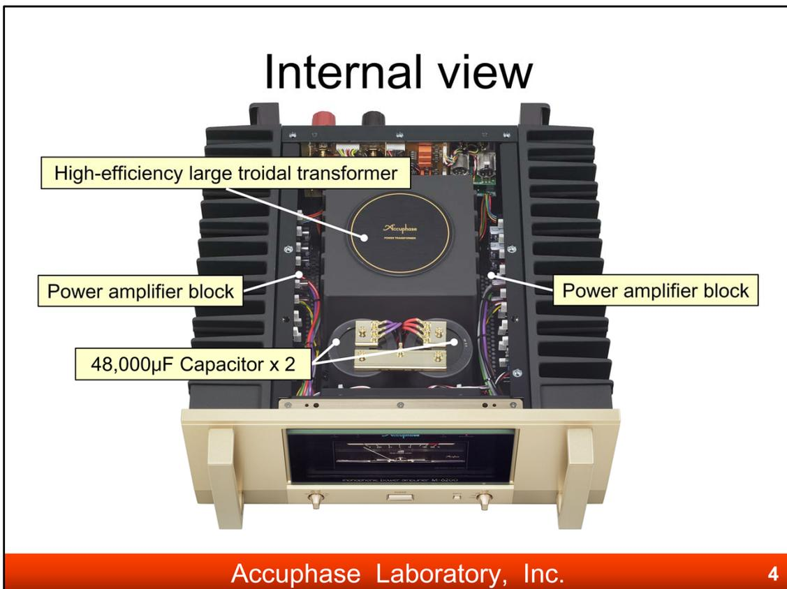
Strong power supply by large Troidal transformer with newly designed heat-radiation fins and a pair of 48,000 $\mu$ F capacitors are installed.
