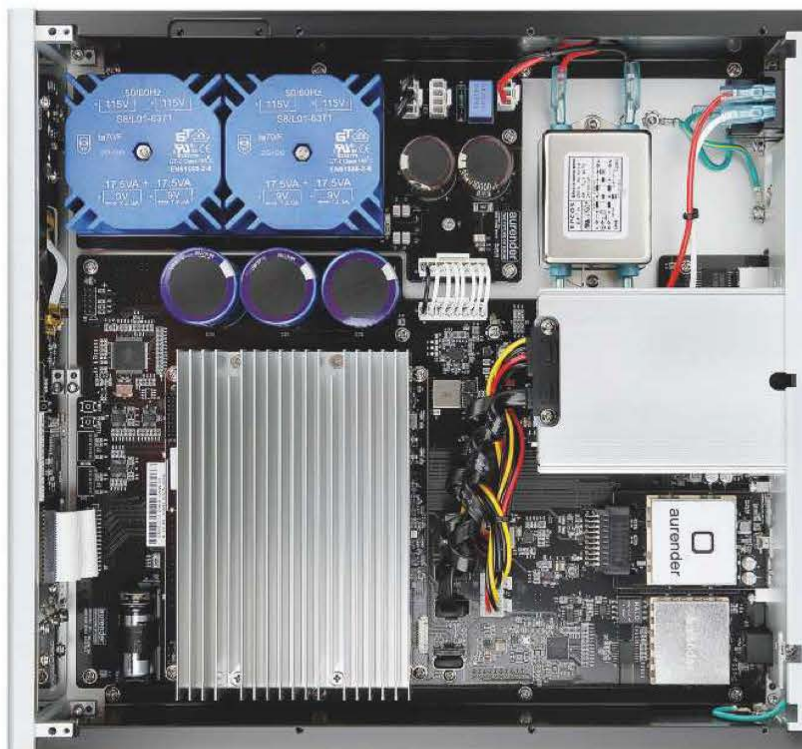
RIGHT: Multiple linear PSUs [top left] serve the Intel Quad Core-based mainboard [under heatsink], 240GB NVMe cache for music playback, and optional SSD/HDD storage [right]. A super capacitor [bottom left] serves as a UPS
