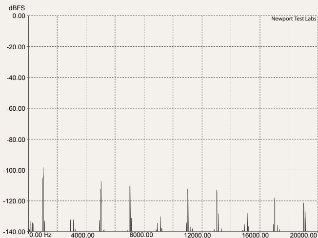
Graph 5: Total harmonic distortion with 1kHz sine wave at -89.46dB. Not dithered. (44.1kHz/16-bit)
