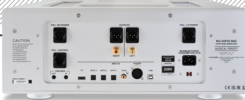
ABOVE: The Nu-Vista DAC offers USB-B (768kHz/32-bit and DSD512), AES/EBU, coaxial and three optical inputs (192kHz/24-bit and DSD64) alongside RCA and balanced XLR outputs. The I 2 S (on HDMI) input is reserved for future use while the five-pin XLR sockets are included to service the outboard Nu-Vista PSU upgrade
