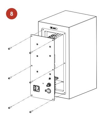
Attach the active crossover module to the back of the speaker using the screws retained from step 1. Initially screw on finger-tight, then secure with a quarter-turn using the hex key.
