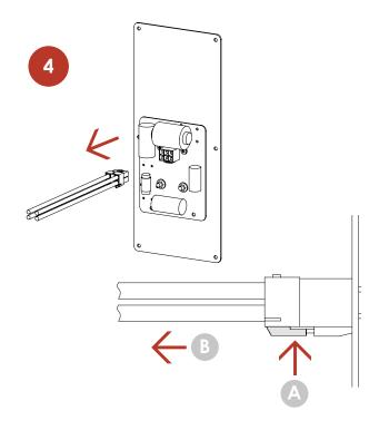
Disconnect the cable from the passive crossover by firmly pressing the connector tab (A) and gently pulling away from the board (B).
