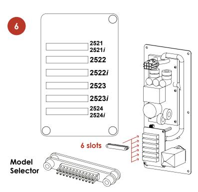
The black circuit board on the new **active crossover** module has 6 slots – one for each model of speaker. Insert the **Model Selector** into the slot that matches your loudspeaker. Ensure the Model Selector is fully seated.
