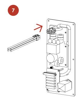
Connect the speaker's internal cable to the active crossover module.
