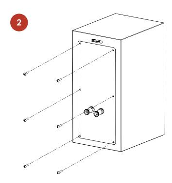
Remove the screws from the existing backplate with the hex key included and retain the screws.
