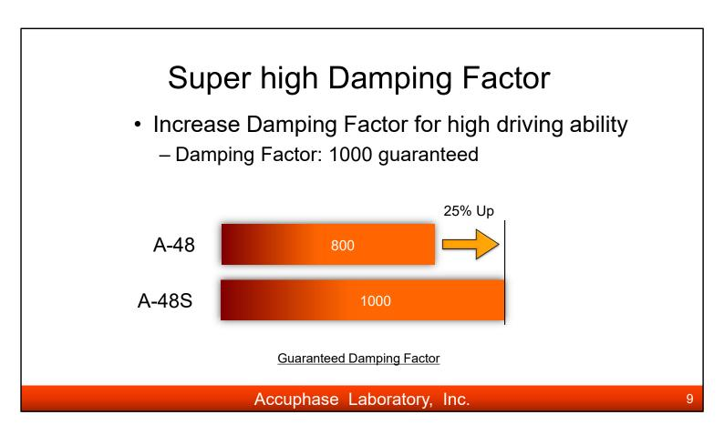
The A-48S achieves 1000 of guaranteed Damping Factor, significantly improved driving capability compared to previous models. This value is the same as the top models A-300 and A-80
