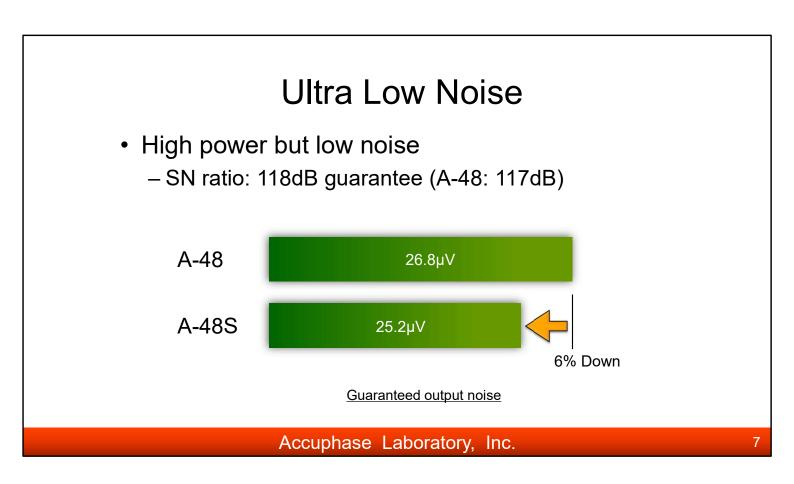
The noise performance of the A-48S is remarkable compared with the former A-48.
