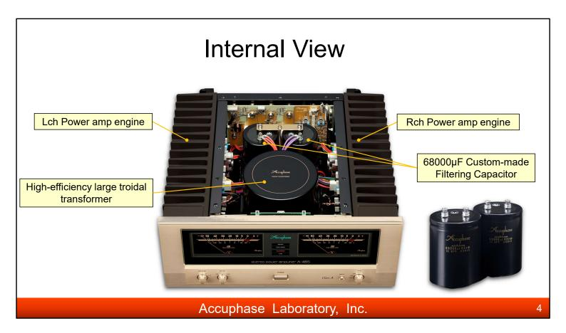
A-48S has a mono-block construction.
