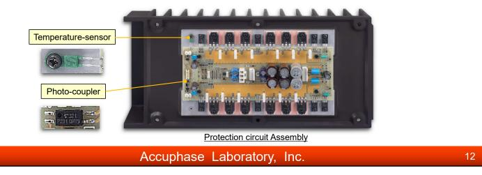
The newly designed output protection circuit can detect any short-circuiting of the speaker terminals with due consideration for product safety.
