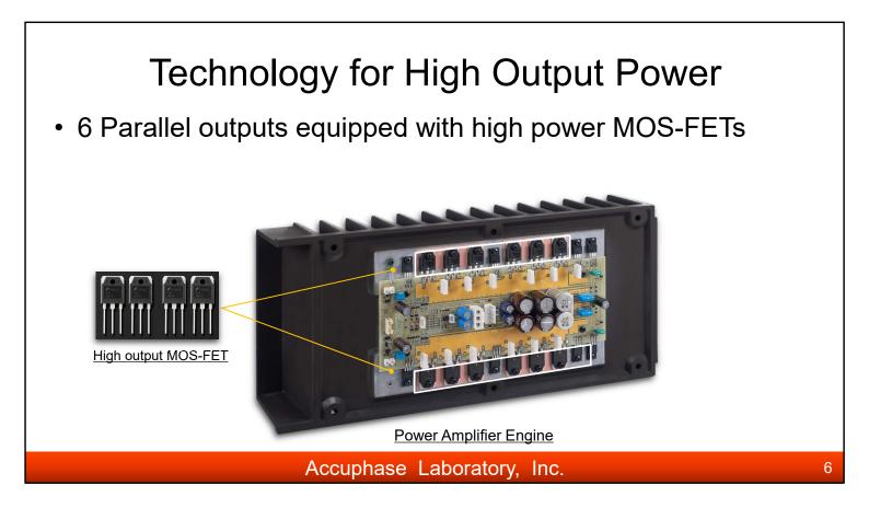
The A-48S power amplification stage uses a 6-parallel push-pull power transistor architecture. By connecting output elements in parallel, the output impedance is lowered to improve the driving capability. And the same time, the load per transistor is reduced and it enables power to be supplied with a margin of safety under all conditions.
