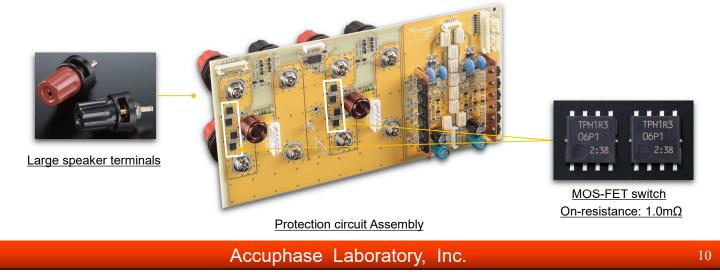
Mechanical relays are the typical components for speaker protection. Still, the contact resistance of mechanical relays is higher than people think.
