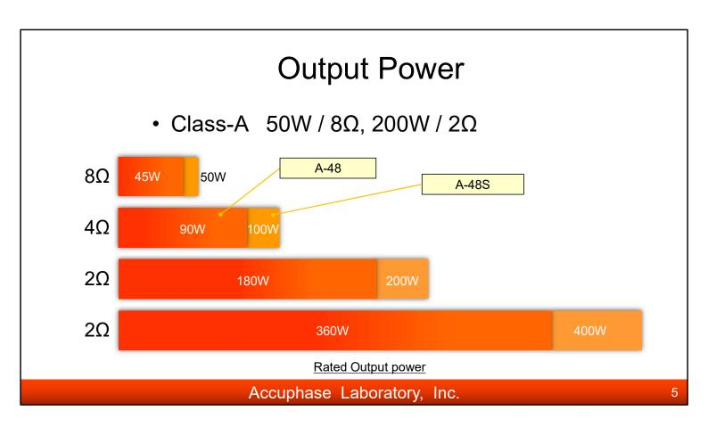
The high-power design provides the rated output power of 50W/8 $\Omega$ , 100W/4 $\Omega$ , and 200W/2 $\Omega$  that vastly exceeds conventional models, securing an overwhelming dynamic range.
