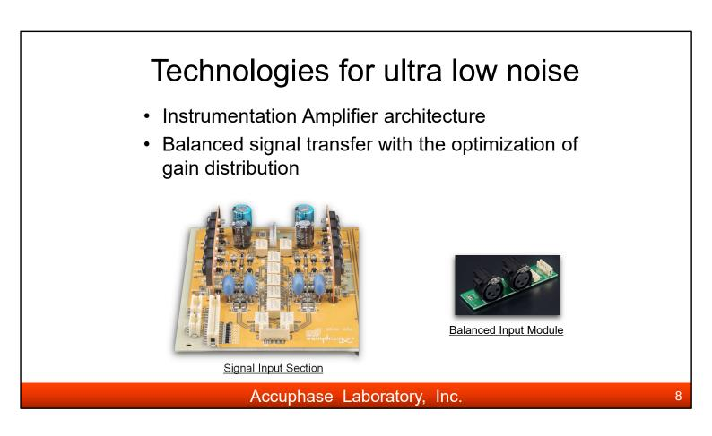
With balanced circuits in the signal input section, the amplification stage entirely comprises an instrumentation amplifier principle that equalizes input impedance on the + and – sides for excellent external noise suppression and provides optimal circuitry for this high-end audio amplifier.
