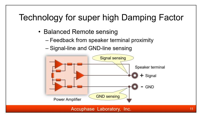
"Remote Sensing" is the technique to lower the output impedance of the amplifier by the negative feedback with a signal sensing from nearby the speaker terminals.
