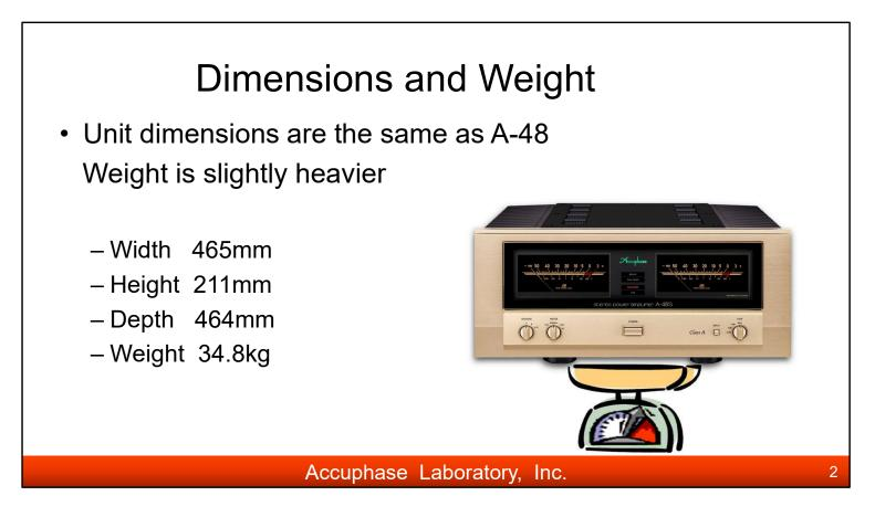
The dimensions of the A-48S are the same as the A-48, and the weight is a little heavier, it weighs 34.8kg.
