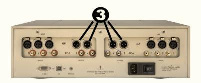
The inner XLR connections on the rear of the Inspiration 2 Preamp are outputs. The signal at these outputs is the same—it does not matter if you use output 1 or output 2. To remove an XLR plug, push on the tab on the connector body and pull the plug out. Be sure to match the output to the correct channel on your amp. Looking at the back of the Inspiration 2 Preamp, the outputs on the left side are for the right channel, the outputs on the right are for the left channel.
