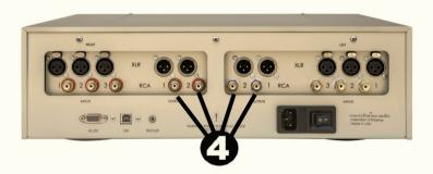
RCA unbalanced outputs are also supplied for amps and recording devices not equipped with XLR jacks. The signal at these outputs is the same—it does not matter if you use output 1 or output 2.
