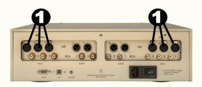
On the rear of the Inspiration 2 Preamp are six XLR inputs, two on each side. As you are looking at the rear panel, the left three XLR inputs are for the right channel, the right three inputs are for the left channel. Underneath each jack is the corresponding input number. Use of XLR connections is recommended for the best possible audio quality. To remove an XLR plug, push on the tab above the jack and pull the plug out.
