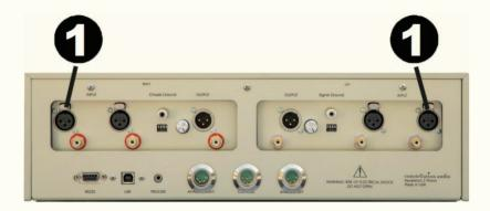
The XLR inputs farthest to each side of the back panel of the Revelation 2 Phono are for use with MC cartridges. As you are looking at the rear panel, the left XLR inputs are for the right channel, the right inputs are for the left channel. These correspond with input MC-1. Use of XLR connections is recommended for the best possible audio quality. To remove an XLR plug, push on the tab above the jack and pull the plug out.
