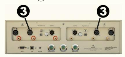
This XLR input is for use with MM cartridges. As you are looking at the rear panel, the left XLR inputs are for the right channel, the right inputs are for the left channel. These correspond with input MM. You may use either the XLR or RCA connection for input MM, but not both. Use of XLR connections is recommended for the best possible audio quality. To remove an XLR plug, push on the tab above the jack and pull the plug out.
