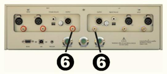
RCA unbalanced outputs are also supplied for preamplifers not equipped with XLR connections. When connecting to an amplifier, be sure to match the output to the correct channel on your amp. As you are looking at the back of the Revelation 2 Phono, the output on the left side is for the right channel, and the output on the right is for the left channel. To remove an RCA plug, grasp it by the connector body and pull the plug out.
