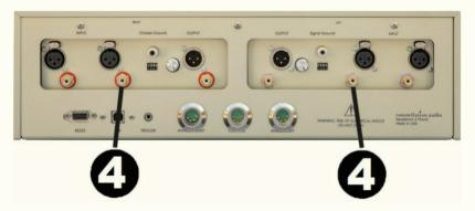
This unbalanced input is provided as a convenience for use with unbalanced signals from MM cartridges. These jacks correspond with input MM. You may use either the RCA or XLR connection for input MM, but not both. Whenever possible, we recommend using XLR connections instead. Connecting to an unbalanced source is handled in the same way an XLR balanced source. To remove an RCA plug, grasp the plug and pull it out. Do not pull on the cable.
