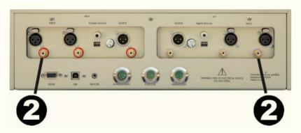
This unbalanced input is provided as a convenience for use with unbalanced signals from MC cartridges. These jacks correspond with input MC-2. Whenever possible, we recommend using XLR connections instead. Connecting to an unbalanced source is handled in the same way an XLR balanced source. To remove an RCA plug, grasp the plug and pull it out. Do not pull on the cable.
