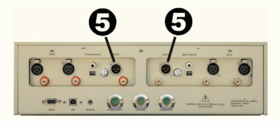
The inner XLR connections on the rear of the Revelation 2 Phono are outputs. To remove an XLR plug, push on the tab on the connector body and pull the plug out. Be sure to match the output to the correct channel on your preamp. As you are looking at the back of the Revelation 2 Phono, the output on the left side is for the right channel, the output on the right is for the left channel.
